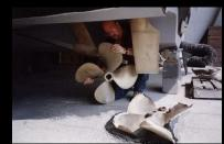
Replacing damaged props and shafts on a 50' Sport Cruiser
